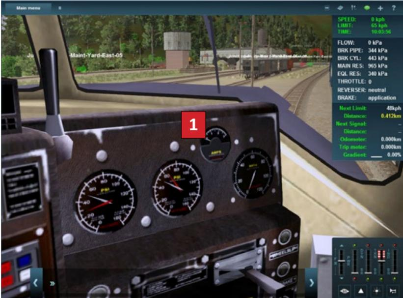
**1** The Load Indicating Meter or Ammeter provides the best guide for throttle handling when accelerating a train. By observing this meter, it will be noted that the pointer moves to the right (increased amperage) as the throttle is advanced. Thus for maximum acceleration without slipping, the throttle should be advanced one notch each time the pointer begins moving back toward the left, until full power is reached in notch 8.
