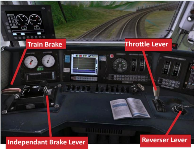
**NOTE** *In-Cab SS4 Locomotive shown. Cab interiors and lever positions vary for each locomotive.*
