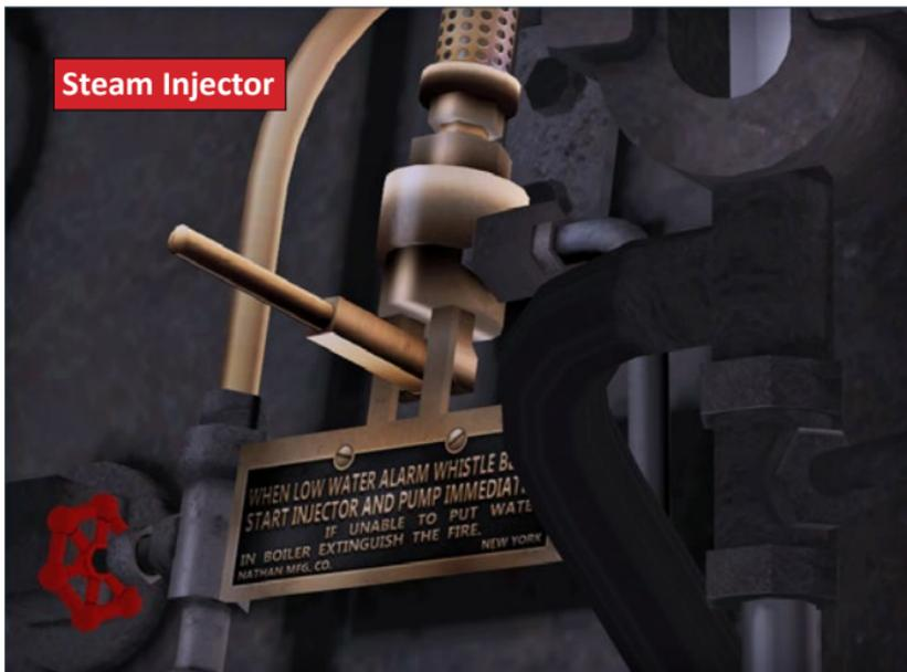
The Steam Injector is a precision piece of equipment which uses a venturi system to use high pressure steam to push water from the tender into the boiler under pressure through a check valve which only allows water into the boiler if the pressure behind the water exceeds the pressure in the boiler.
