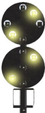
On densely used track or where line speed is high, a fourth aspect (Advanced Caution) may be used to give advance warning to trains that they have to slow down.
