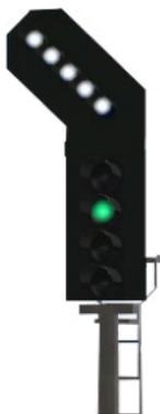
This signal is showing the left hand diverging Route is set. It doesn't specify how fast the junction should be taken - in this case this information would be given by a separate speedboard with a left hand arrow on it near the junction.
